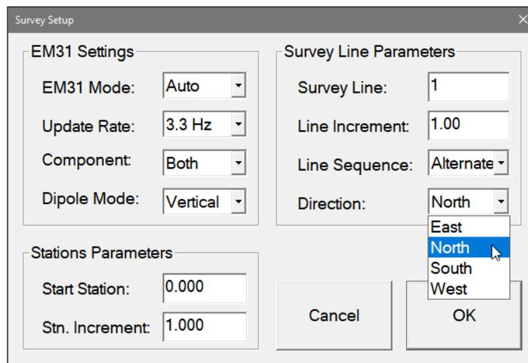
This screenshot is identical to the previous one, but the 'Direction' dropdown menu is expanded. The options listed are North, East, North (highlighted in blue), South, and West.
