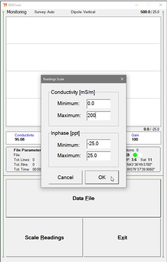
and top right corners of the plot area. The first numbers indicate scale for conductivity and the second (following slash) numbers are associated with Inphase scale. Values displayed in bold indicate the scale that is associated with grey grid lines.
