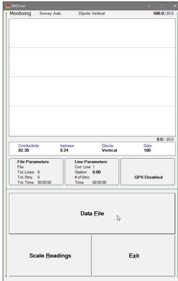
One line of text in the top section provides survey parameters (used in Stand By and Logging modes) and instrument information. In Monitor mode this section displays: current logging session mode (Monitor, Stand By or Logging), survey mode (Auto, Wheel, Manual), and user specified instrument dipole mode (Vertical, Horizontal, or Both). When fiducial marker is pressed then label **Marker** is displayed.
