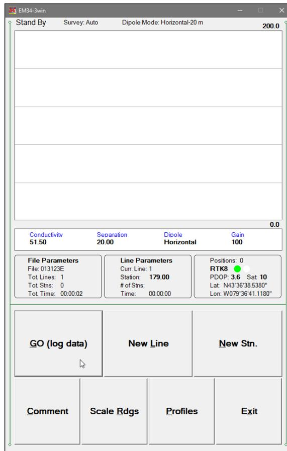
The main portion of the screen is occupied by the plot area which displays profiles (see Figure below which shows Stand By mode after some data were collected). Scale for conductivity is labeled at the top and bottom of the plot window. The amplitude scale is divided by three to five grey grid lines. In the case where the amplitude scale starts with a negative value, then the grid line corresponding to zero is always plotted as a thicker line.
