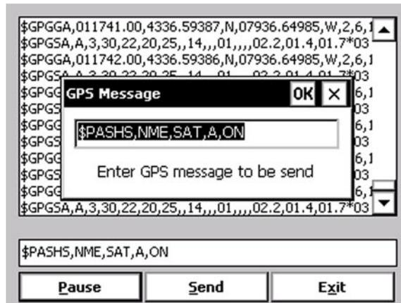
After this command is received by the GPS receiver, the confirmation message will be sent by the receiver (\$PASHR, ACK\*3D) and data stream will contain the message SAT (\$PASHR, SAT,..... in the above figure).
