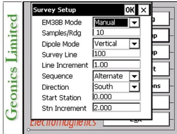
This parameter describes number of readings that will be taken after the trigger switch is pressed. At the end of sampling time the logger will beep and an average value will be written in to the file and plotted on the screen. During the sampling period interval data are measured at approximately 10 readings per second. For example by specifying 10 samples, 1 second will be used at each station. The maximal sampling is 100 readings which corresponds to approximately 10 seconds at each station.
