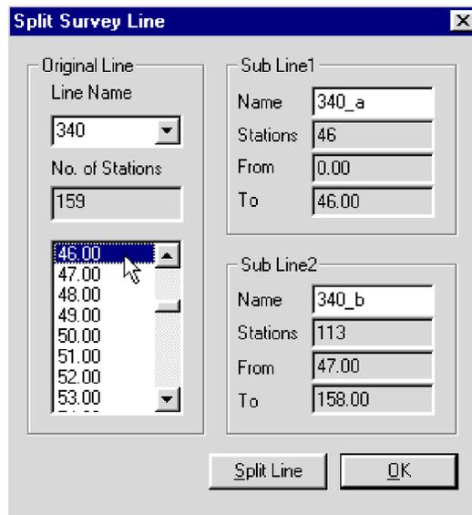
Figure 6.7: Selecting the station in the line
