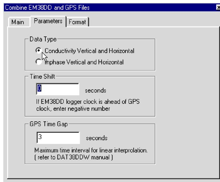
**Figure 8.6: Parameters page in the Combine EM38 and GPS Files window**
