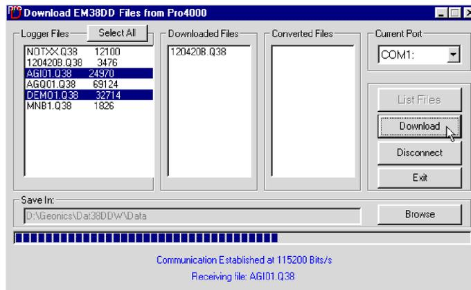
**Figure 3.19:** Download window during data transmission
