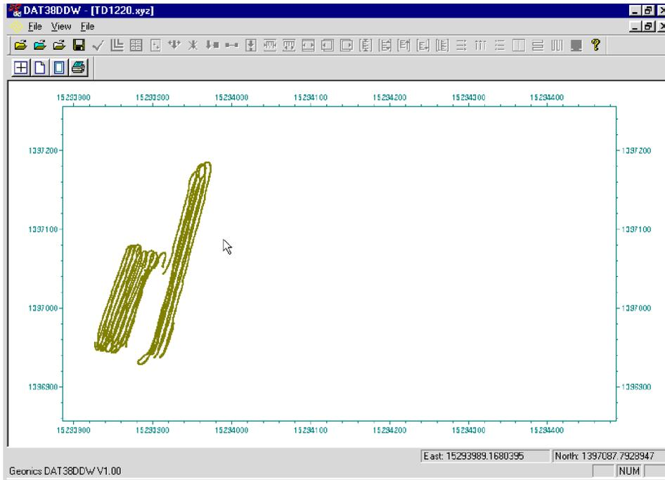
**Figure 8.11:** Layout of survey as created in the XYZ output file
