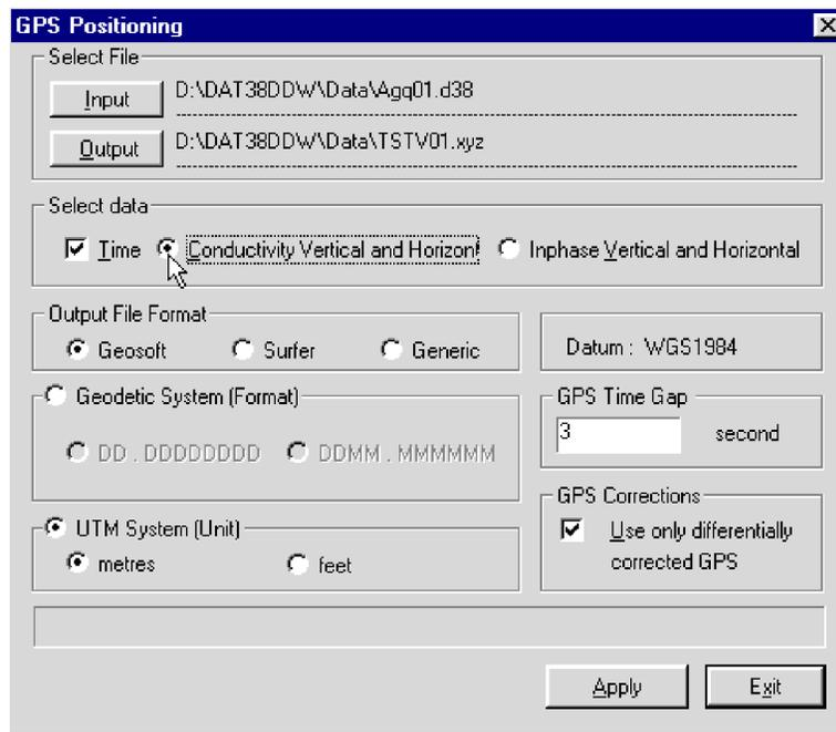
*Figure 8.15: GPS Positioning window with selected Input and Output files*
