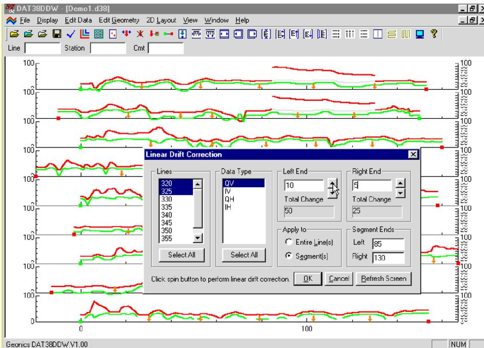
Figure 5.11: The DAT38DDW during Linear Drift Correction of Line Segments
