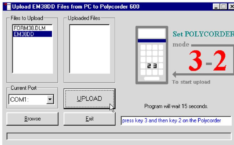
Figure 3.4: Upload File window waiting for Polycorder entry
