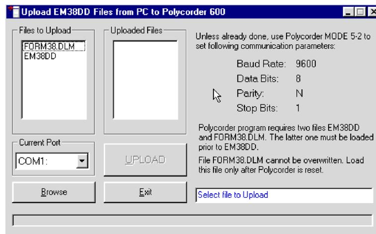
Figure 3.2: Upload EM38DD Files to Polycorder 600 window
