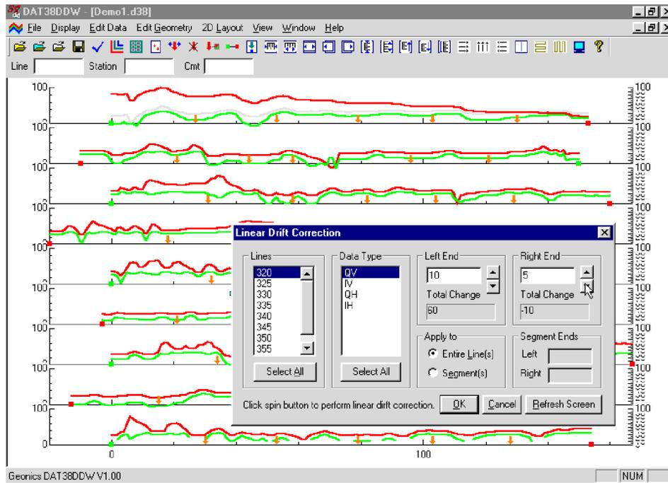
Figure 5.10: The DAT38DDW during Linear Drift Correction for the Entire Line
