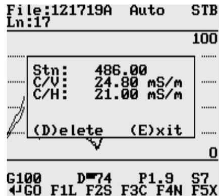
This function allows operator to delete previously recorded reading(s). The reading (station) to be deleted is displayed on the screen. The data will only be deleted when the key **D** is pressed. The program will then display the next previous station, and allow it to be deleted in a similar fashion. If there is no further data available, the program will provide related information.
