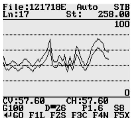
The main portion of the screen in graphic mode is occupied by the plot area. Readings in the plot area can be displayed in the user specified scale. The amplitude scale is divided by four or five dotted grid lines. In cases where the amplitude scale starts with a negative value, then the grid line corresponding to zero is always plotted as a solid line.
