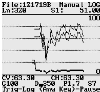
There is only one option available in the Logging mode - pause logging. After a Pause key (any key, Alt+F1, or Ctrl+F5) selected in Logger Setup menu is pressed the recording is stopped and the Log Data menu returns to the Stand By mode. The EM38DD data will be displayed with the update rate approximately 10 readings per second, however data will not be saved in the log file, audible click will stop if Sound option was enabled, and if graphic mode is used, profile curves will not be updated.
