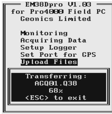
Transferred files (in EM38Dpro format) will be displayed in the centre list box. After the transfer of all selected files is complete, files in the EM38Dpro format are automatically converted to the DAT38DD format (with extension name D38). Converted files will be displayed in the Converted Files list box (see Figure below). Converted files (with extension name D38) can be loaded and processed further in the program.
