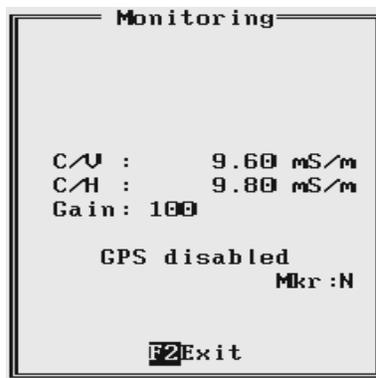
The EM38DD readings are updated approximately 10 times per second during monitoring session. If **Quad-phase** was selected on the instrument panel values of conductivity in mS/m are displayed, and when **Inphase** was selected values of the measured Inphase component in ppt will be given. The instrument scale, and state of fiducial marker are continuously updated.
