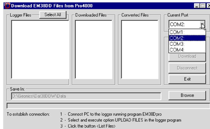
To start downloading the data files, connect the field computer (Pro4000) and PC computer with the serial cable.
