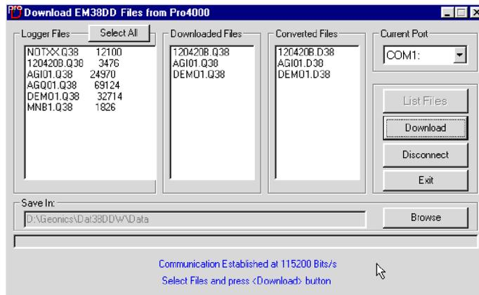
Click the **Disconnect** button to cancel communication with logger. The Download EM38Dpro Files from Pro4000 window will remain on the screen and next data transfer session (i.e. from another logger) can be performed. Clicking the **Exit** button will stop Data Transfer function and the Download EM38Dpro Files from Pro4000 window will disappear.
