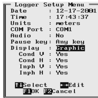
Parameter **Cond V** (conductivity in vertical dipole mode), **Cond H** (conductivity in horizontal dipole mode), and similarly for Inphase component **Inph V** and **Inph H** allow you to enable (Yes) or disable (No) display of each type of reading separately.
