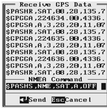
After this command is received by the GPS receiver, the confirmation message will be sent by the receiver (**\$PASHR,ACK\*3D**) and data stream will not contain the message **SAT** (**\$PASHR,SAT,....** in the above figure).
