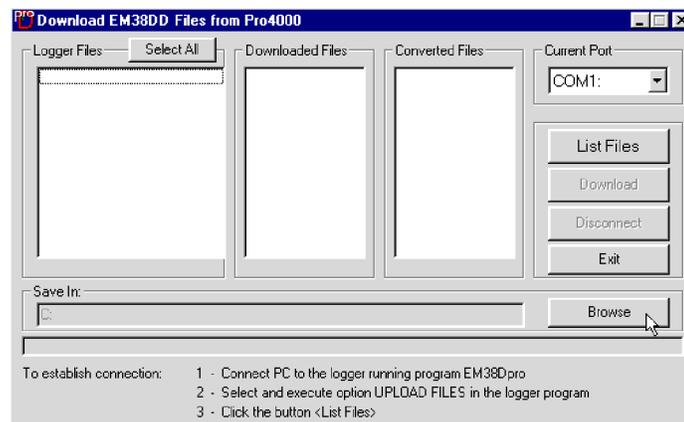
The Download window has three list boxes. The first from the left, labeled Logger Files will contain, after the **List Files** button is clicked, a list of data files located in the field computer and available
