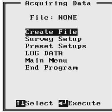
At the top of the screen the current name of the data file is displayed. If data file is not created its name is displayed as NONE. The menu contains several options listed below.
