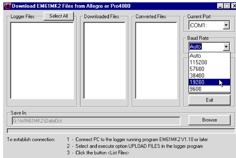
Figure 3.5: Selecting Baud Rate for selected serial port
