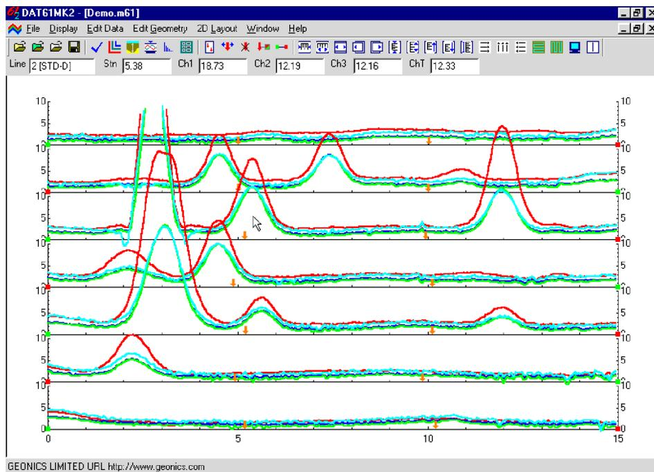
*Figure 4.28: DAT61MK2 screen with data displayed in compressed amplitude mode*
