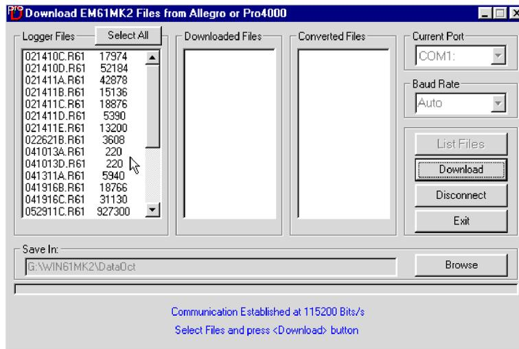
Figure 3.7: Download EM61MK2 Files window after logger files are listed
