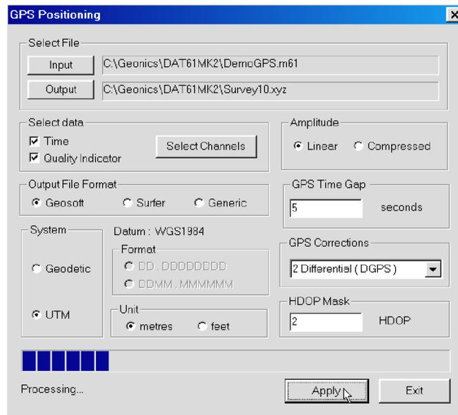
Figure 8.18: GPS Positioning window during creating XYZ (output) file
