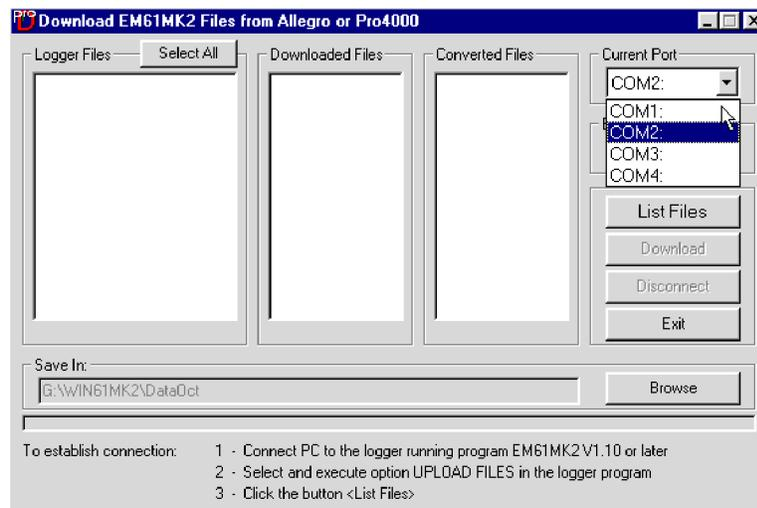
*Figure 3.4: Selecting current serial port number*
