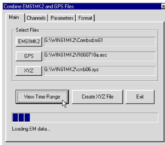
Figure 8.9: Combine EM61MK2 and GPS Files window during reading of EM61MK2 and GPS files
