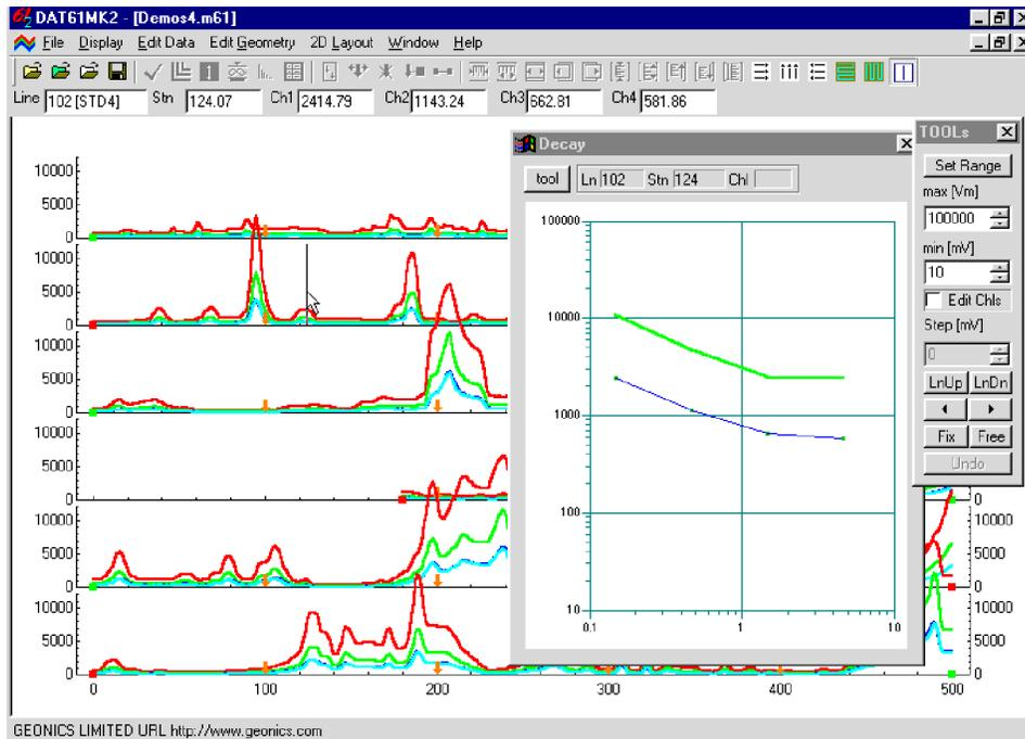
Figure 4.33: Decay window with Fixed decay curve
