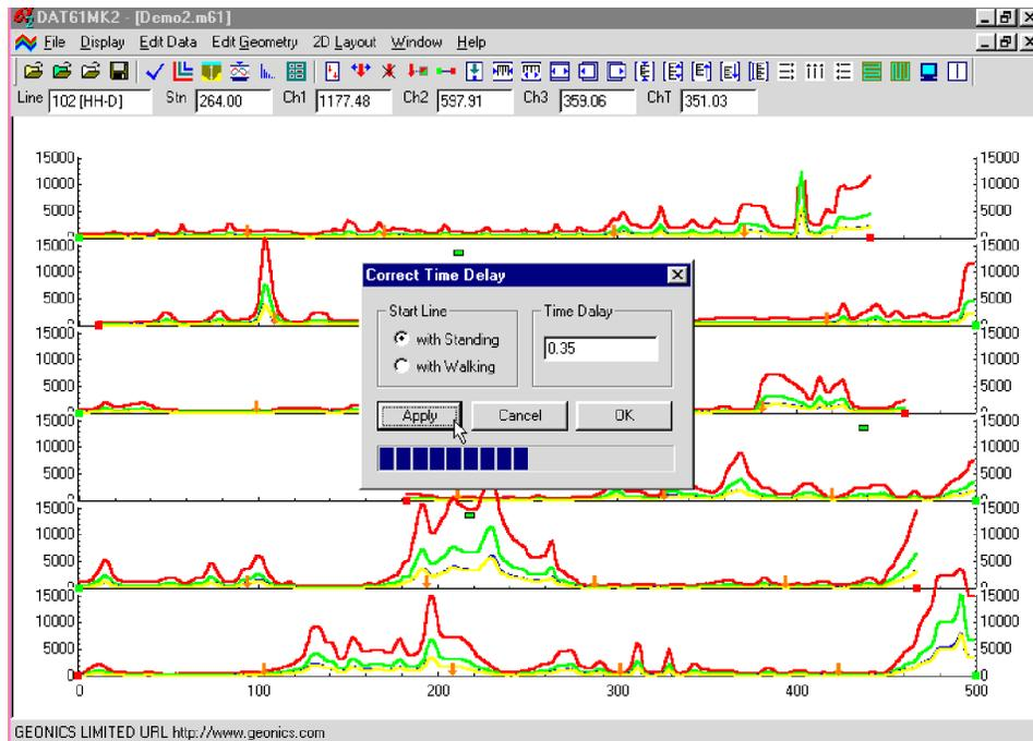
*Figure 6.21: DAT61MK2 screen during Time Delay Correction*
