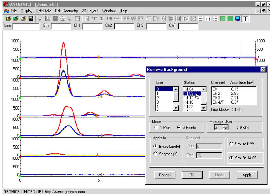
Figure 5.10: The Remove Background window in Two Points Method
