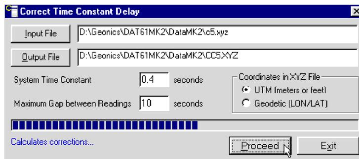
Figure 8.24 Correct Time Constant Delay window during creating corrected XYZ file
