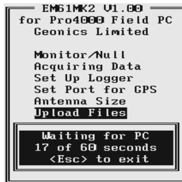
Figure 3.6: Logger Screen during Uploading Files
