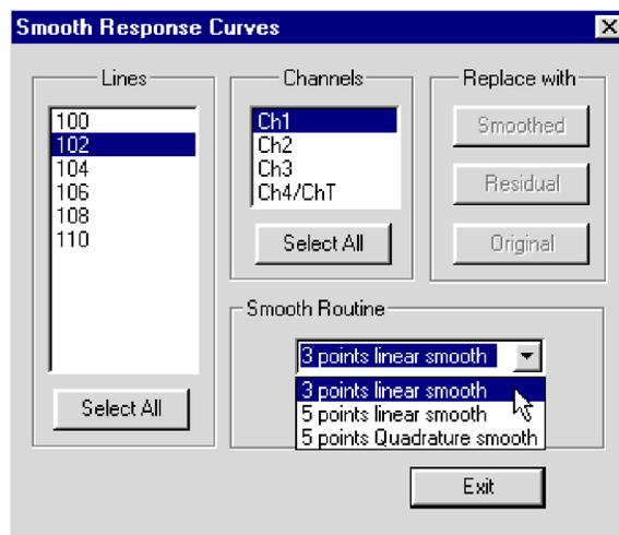
Figure 5.12: The Smooth Data window with list of available smooth functions.
