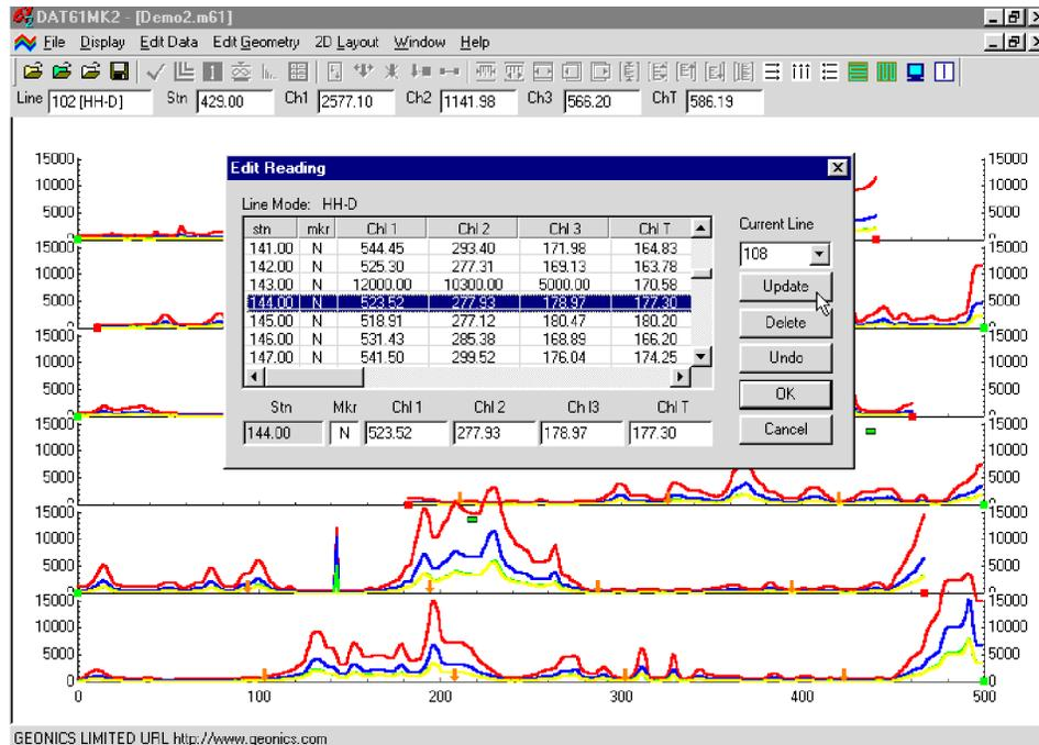
Figure 5.6: Edit Readings window during editing value of channels
