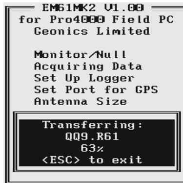
*Figure 3.10: Logger Screen during Uploading File*
