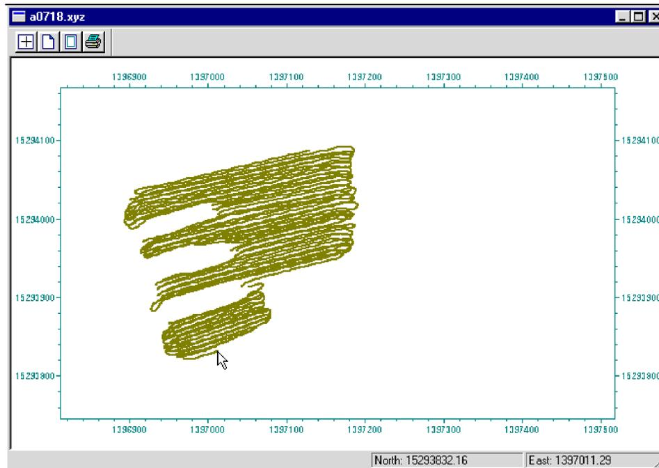
*Figure 8.12: Layout of survey as created in the XYZ output file*
