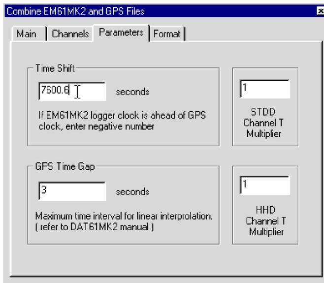
Figure 8.7: Parameters page in the Combine EM61-MK2 and GPS Files window
