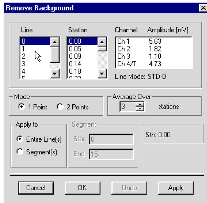
Figure 5.9: The Remove Background window in One Point Method
