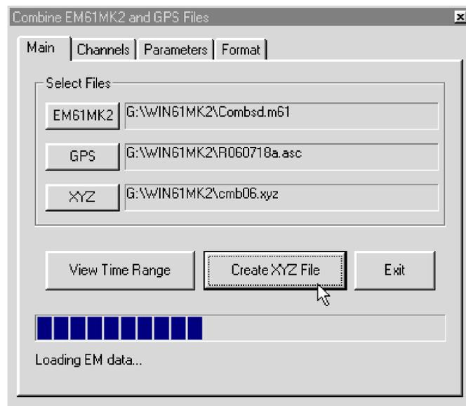
*Figure 8.11: Combine EM61MK2 and GPS Files window during reading data files and creating output XYZ file*
