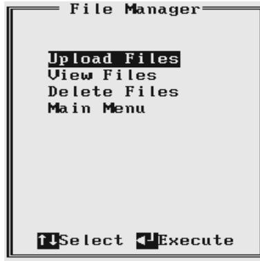
Three options Upload Files, View Files, and Delete Files are described in following sections 14, 15, and 16. Select and execute option Main Menu to return to the main menu of the EM61MK2A.
