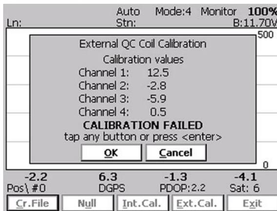
Regardless of the test result (OK or FAILED) the readings will be saved on screen. The program returns to Monitoring window after any button is tapped or ENTER key is pressed. Then the Internal QC coil calibration process can be repeated.
