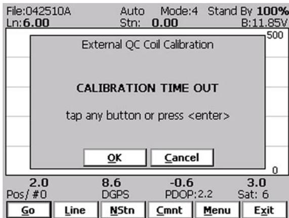
After pressing any key the program returns to Stand By mode window. To repeat External QC coil calibration please repeat the procedure.
