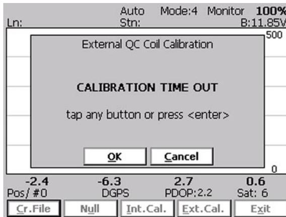
The logger will determine if the instrument has passed test. If after activating the QC coil, the program determines that the reading is inside the standard values within +/- 10% tolerances then a message “CALIBRATION OK” will be displayed.
