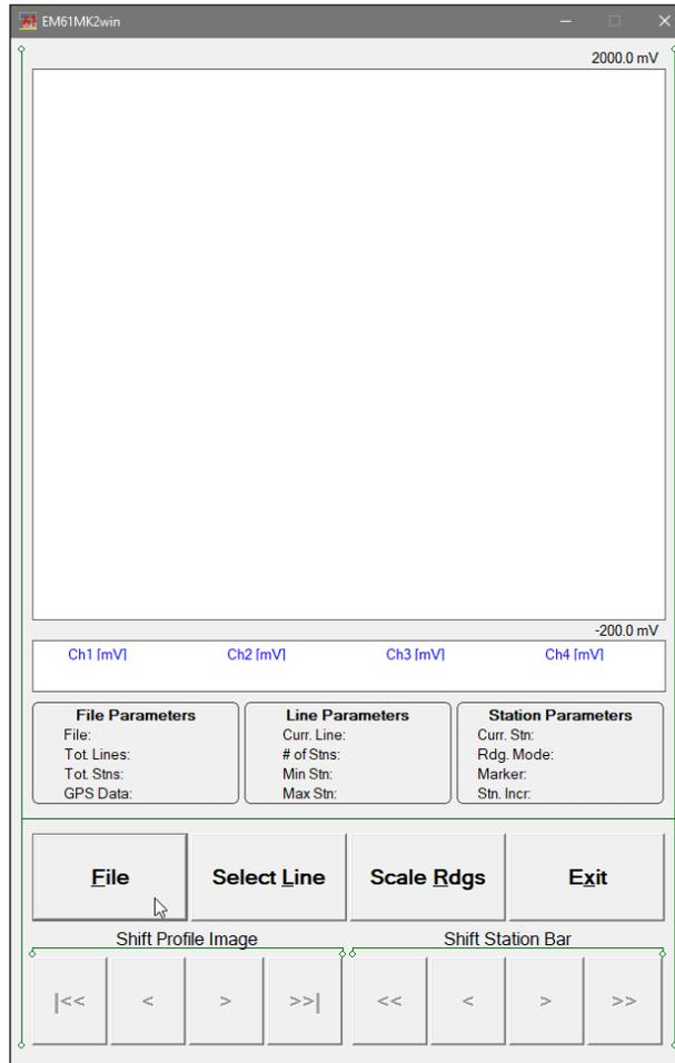
To open the data file click or tap on the button labeled File or execute this option using the keyboard (navigate to the button by pressing TAB key and when highlighted press ENTER key, or use shortcut - press key F). The Open Data File dialog is presented below.
