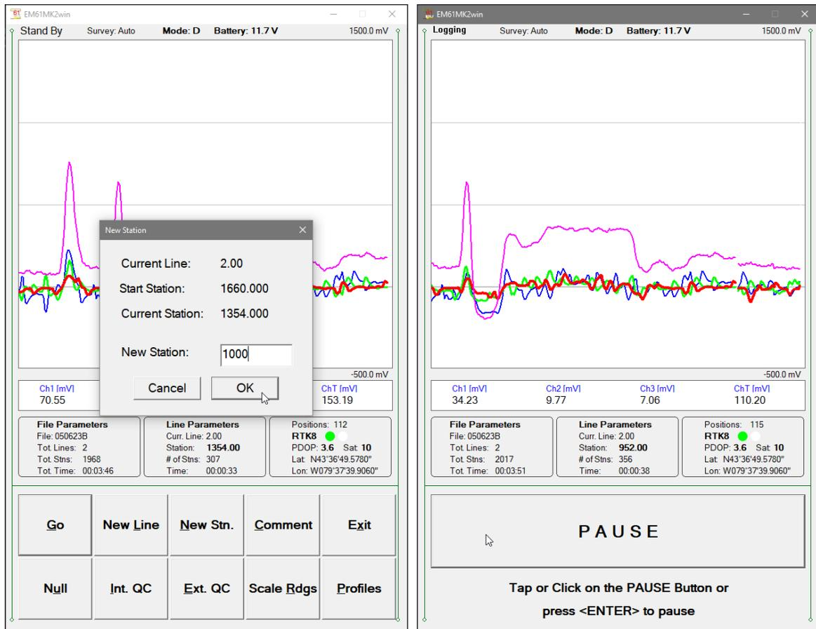
Click on the button **OK** or press **ENTER** key to accept the new value. The program will return to the Logging window in Stand By mode. Current station (**Station:**) value will be updated and after data logging is activated the profile curves will have a small gap (two pixels) showing the new station entry (see Figure above on the right).
