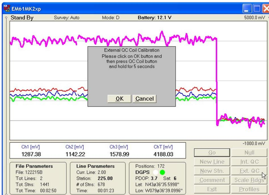
*When External QC Coil Calibration window is displayed please use keyboard keys (O or C) rather than a mouse to execute buttons labeled OK and Cancel. Clicking on buttons by mouse will work, however several mouse button clicks may be required.*
