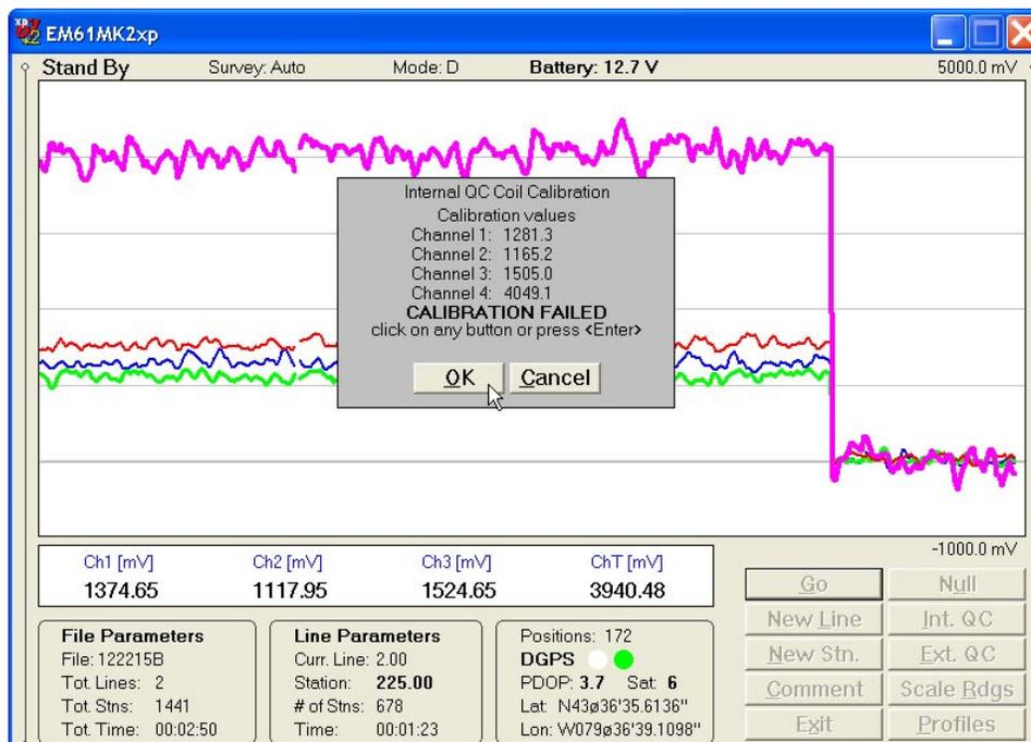
After pressing any key the program returns to Monitoring window. To repeat Internal QC coil calibration please click on the **Int. QC** button again.
