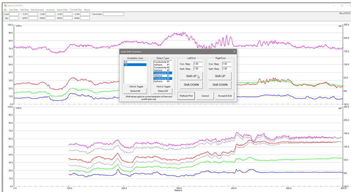
Figure 4.5 DAT38-4 during Linear Drift Correction procedure
