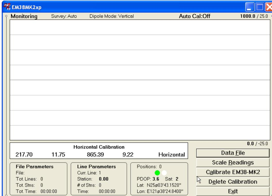
If for any reason the calibration is not successful a proper message will be displayed. Horizontal calibration takes normally 2 seconds and when the procedure is completed a confirmation message will be displayed (Figure below).
