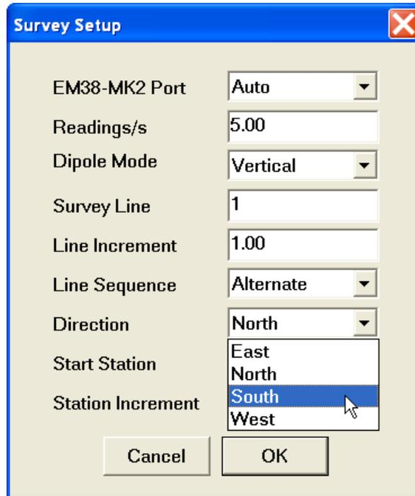
This parameter indicates the heading of the survey line.
