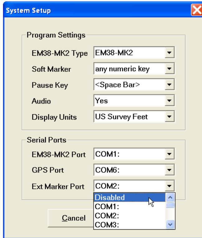
This port must be different than the port specified in the Set Port for GPS option (see next chapter), otherwise a message will be displayed and the ports will have to be reassigned. If External Marker is located on the Extender Arm then The EM38-MK2 and Ext. Marker Port must be the same.
