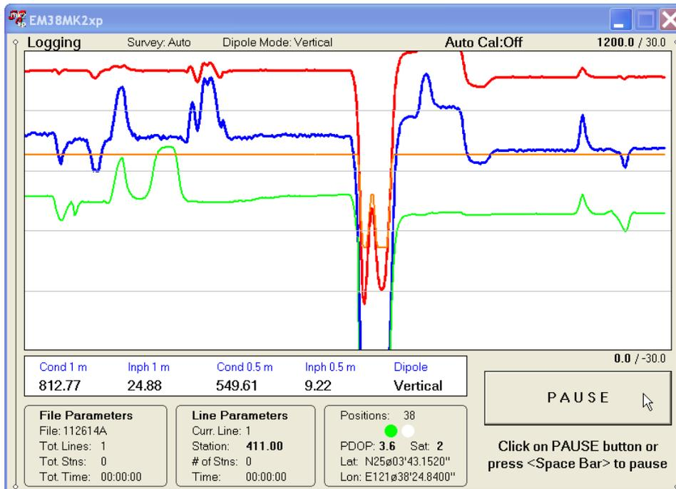
After the screen changes to Logging mode the current station (label **Stn:**) is updated according to the station interval. Similarly, if GPS Input was enabled, total number of GPS positions (label **Positions**) in the data file is incremented every time (usually once a second) GPS position is written to the file. Profile curves (for channels selected in Display Options window) are updated after each reading is written to the data file.
