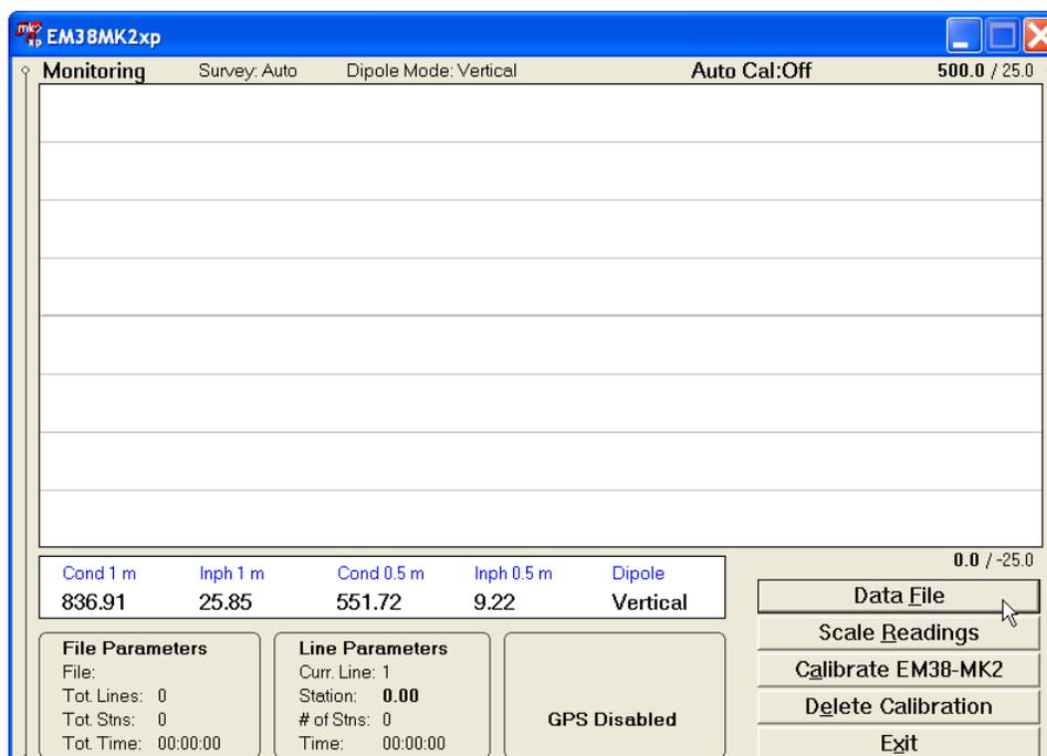
The EM38-MK2 readings and dipole mode are displayed from the left in order: conductivity and Inphase for 1.0 m coil separation, then conductivity and Inphase for 0.5 coil separation, followed by dipole mode (Vertical or Horizontal). Displayed values are labeled: Cond 1 m, Inph 1 m, Cond 0.5 m, Inph 0.5 m, Dipole. Conductivity values are displayed in mS/m and Inphase values are given in ppt. The EM38-MK2 readings are updated approximately 21 times per second during the monitoring session.
