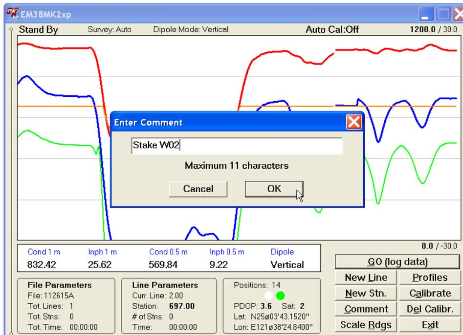
Click on the button **OK** or press **ENTER** key to accept the comment entered in a text box of the dialog. The text of the comment is saved in the file with a corresponding time stamp and the program will return to the Logging window in Stand By mode.
