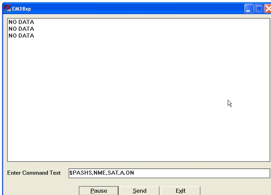
serial port number not correctly specified in Set Port for GPS dialog, GPS receiver not sending any data, and not working or not connected GPS receiver. If the message is updated more often than 7 seconds (i.e. every 1 or 2 seconds) or the display does not show legible characters, it is possible that
