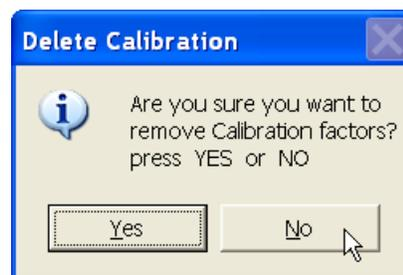
Please confirm by tapping button **Yes**, or pressing Key **Y** or Enter (if button **Yes** is highlighted) to delete (reset) calibration factors. After this is done readings displayed by the instrument console and the logging computer should be similar.
