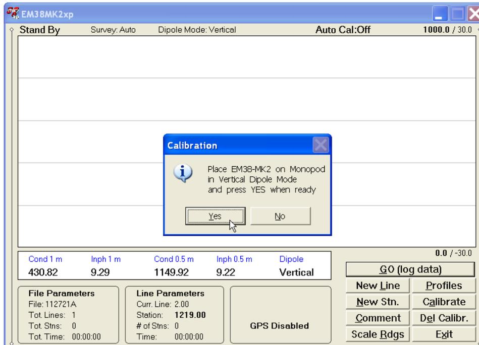
Calibration procedure is the same as described in chapter 6.1 (Monitoring Mode). Please refer to above section of the manual and follow all prompts that appear on the display. Calibration factors will be written to the data file and displayed readings will be adjusted immediately after the Calibration procedure is completed.
