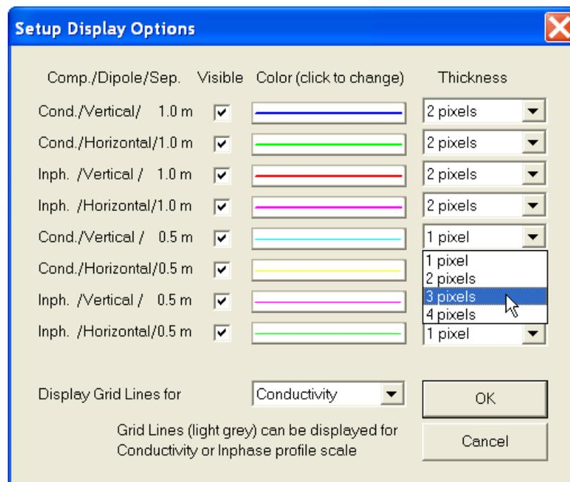
Profiles for both components share the same graphic window, however each component has its own scale. This option allows you to select grid lines to be displayed (as thin grey lines) for conductivity or Inphase scale.
