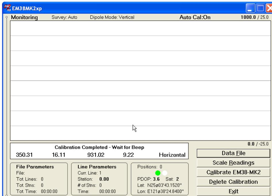
After beep the above message disappears and program returns to normal operation. All calibration factors are saved in the field computer memory and will be used in consecutive program runnings. Unless a new version of the program is loaded the only possibility to delete (or reset to zero) calibration factors is using option Delete Calibration.
