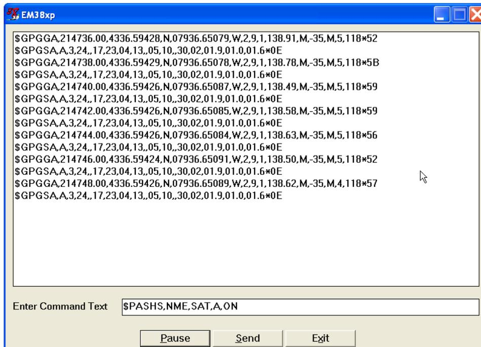
sage transmitted by GPS receiver will appear in the top portion of the display (the end may be cut off if an NMEA message is longer than screen). The display is updated with the frequency the GPS receiver outputs data. This allows you to recognize the GPS update rate and type of messages being sent by the connected GPS. In cases where the GPS data is not received by the logger a message NO DATA and current time will appear in the top window of the display, as shown below.
