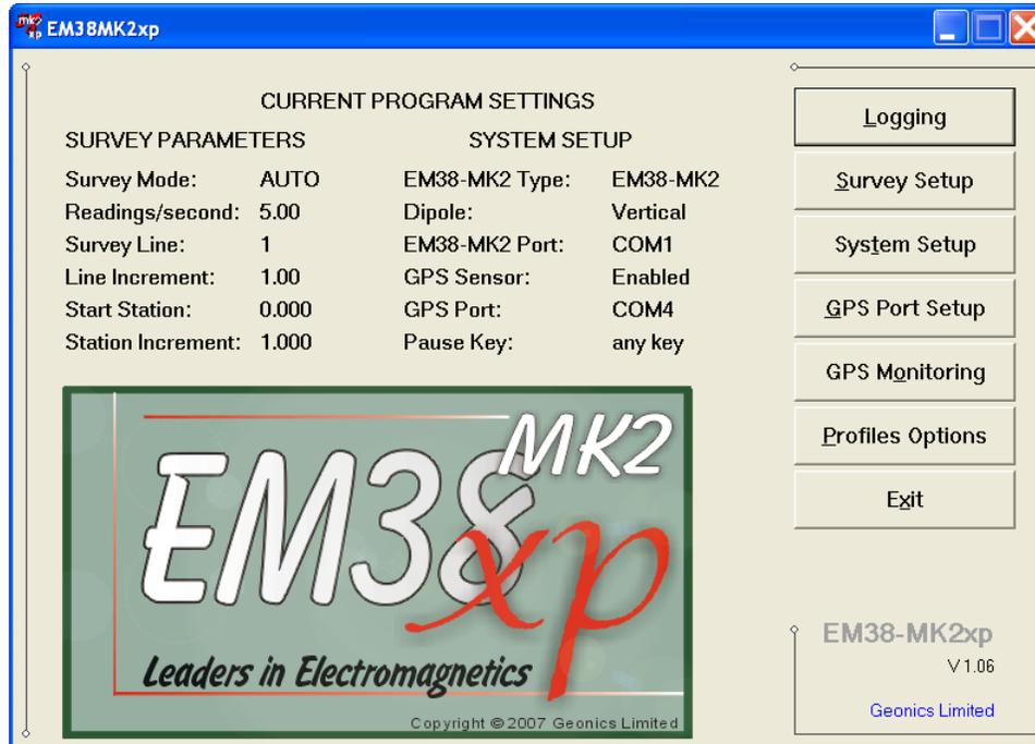
The EM38MK2xp is a command button and dialog driven program. Command buttons can be executed by clicking with the left mouse button, or by pressing the indicated (underlined) character on the keyboard, or by using TAB to scroll through the buttons and ENTER to execute. In the Main Screen of the program Up and Down arrow keys can be also used to scroll through the buttons.
