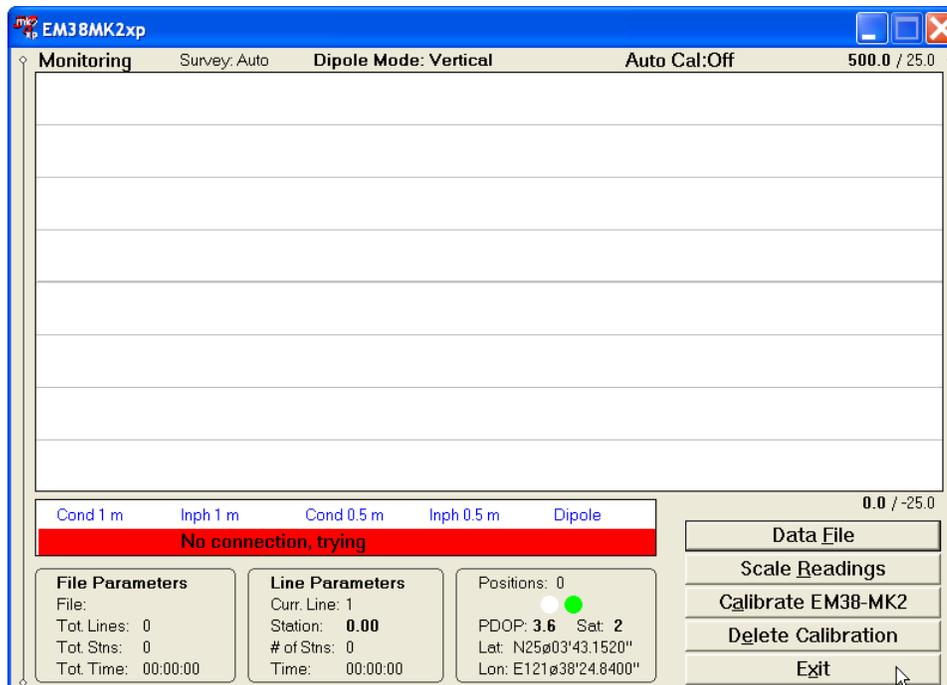
also state of Auto Calibration (ON or OFF). When fiducial marker is pressed then the label **M** is displayed.
