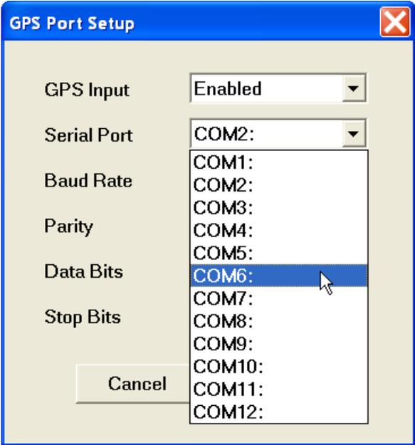
MK2), otherwise a message will be displayed and ports will have to be reassigned. Clicking on the down arrow next to the text box labeled Serial Port opens a drop-down box showing the available ports, or when the keyboard is used activate the text box by pressing TAB key and then by using up or down arrow keys select one of available items.
