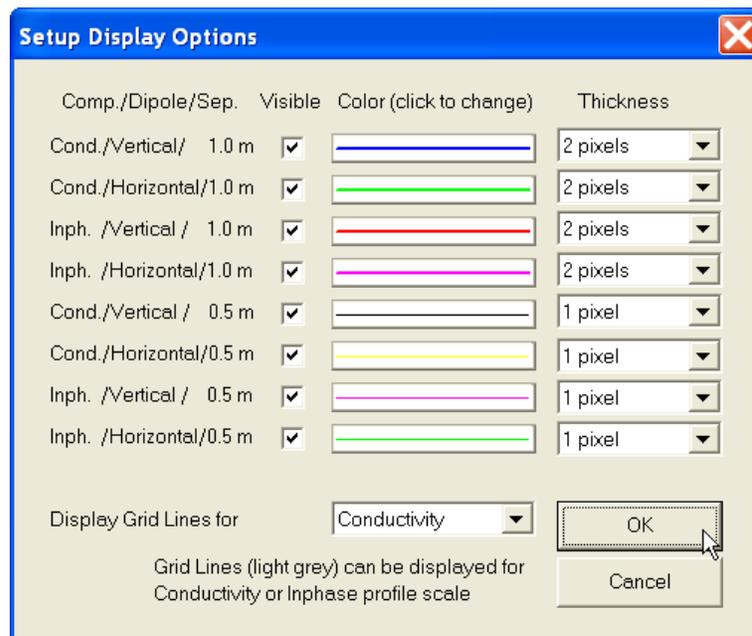
Please refer to chapter 5 where this dialog and its parameters are described in detail. Click on the button **OK** or press **ENTER** key to accept updated display parameters. The dialog will disappear and profile plot area will be redrawn in Stand By mode. To return to Stand By mode and current display options (state before this dialog was selected) click on the **Cancel** (X) button or press **Esc** key, the dialog window will disappear.
