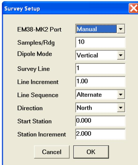
This option could be used to improve quality of data in areas of high industrial noise, especially if the ground conductivity is relatively low (small response signal).
