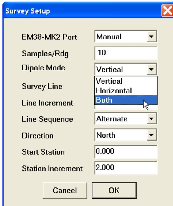
When Manual mode was selected three settings are available: Vertical, Horizontal, and Both. If Auto or Wheel mode was selected two available dipole modes are: Vertical or Horizontal.
