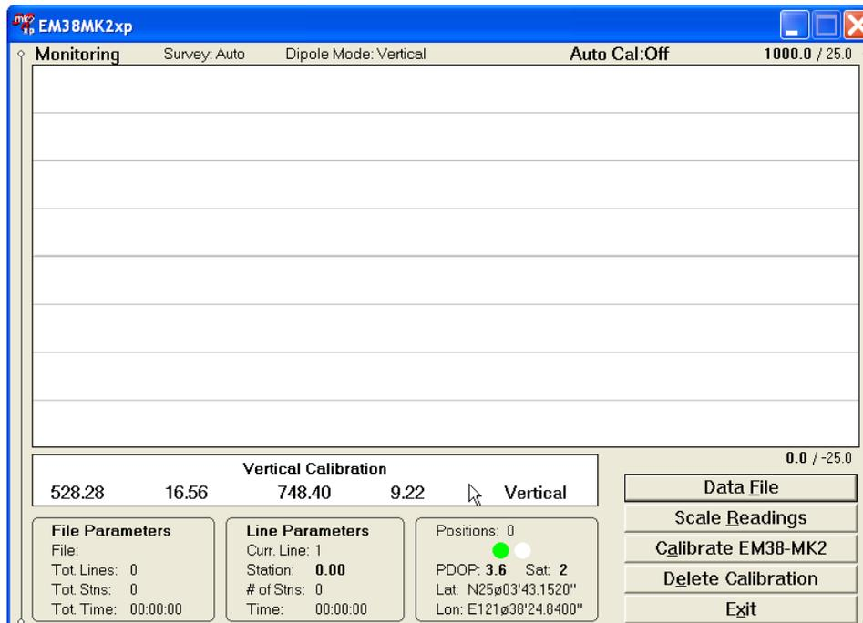
After the Vertical calibration is completed (usually few seconds) the program will beep and a message **Rotate to Horizontal mode within 60 seconds** will appear.
