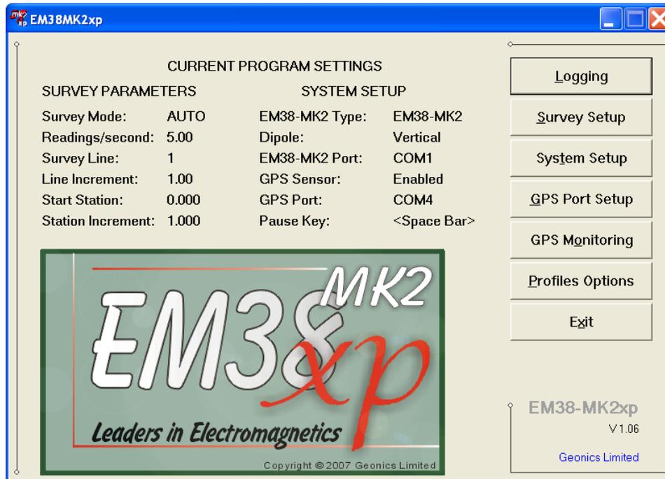
and a data file can be created. The instrument can be also calibrated in Monitoring mode. After a data file is created in Monitoring mode, the program switches to Stand By mode and allows access to Logging mode. In Stand By mode instrument output can be monitored and some survey and logging parameters can be changed, and the Logging mode is used only to record data. Two modes Stand By and Logging are toggled by **GO** and **Pause** buttons.
