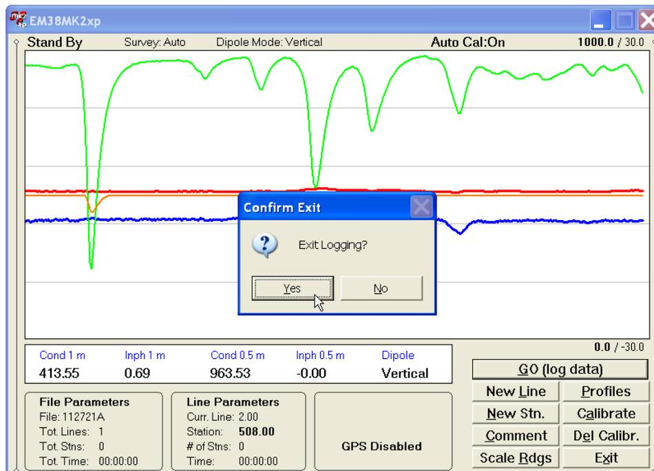
After the above message is confirmed the program stops logging, closes the data file and returns to the Main Screen.
