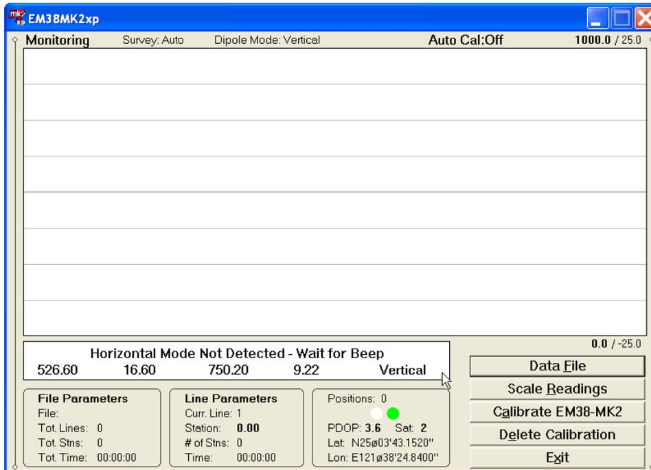
The program monitors instrument orientation and as soon as it detects that the EM38-MK2 is in proper position it will display the following message: **Preparing for Horizontal Calibration**. After a small delay required for stabilization the Horizontal Calibration will be performed.
