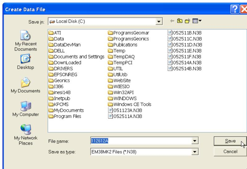
The file name can be specified in the Create Data File dialog using the Windows standard interface procedure. The EM38-MK2 data files cannot be appended.
