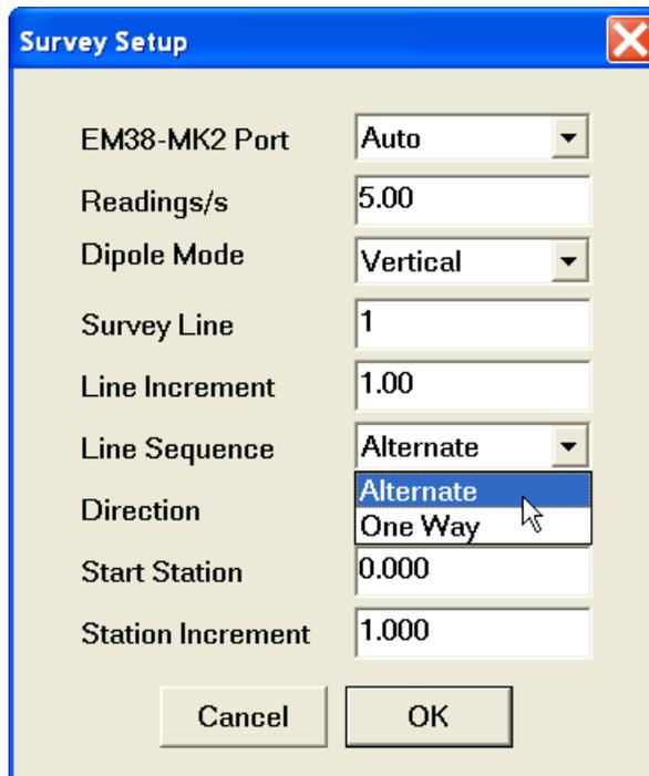
The choice of this parameter will affect the default start station, a signature of the station increment, and line direction when parameters for the next survey lines is determined.
