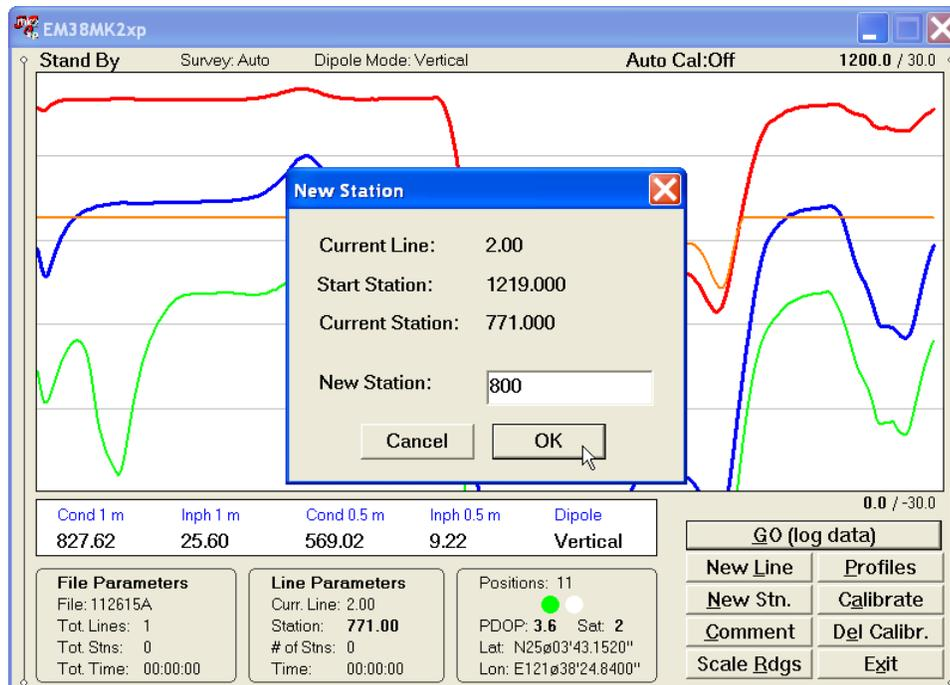
updated and after data logging is activated the profile curves will have a small gap (two pixels) showing the new station entry (see Figure below).
