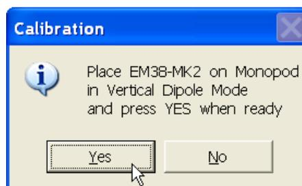
After the instrument is placed on the monopod in Vertical dipole mode click on the button **Yes** or press key **Y** (or **Enter** if button is highlighted). After button **Yes** was clicked a messages box disappears and a prompt **Vertical Calibration** is displayed. From now on all messages and prompts will be written under plot section of the screen, in a line that is normally used to display labels for EM38-MK2 readings.
