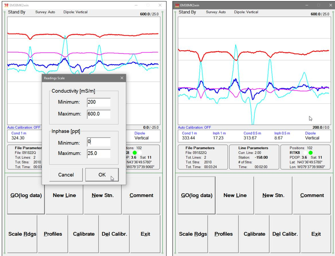
bold indicate the scale that is associated with grey grid lines. After minimum and maximum values are specified click on the button **OK** or press **ENTER** key to accept new values and the profile plot area will be redrawn (see Figure above on the right).
