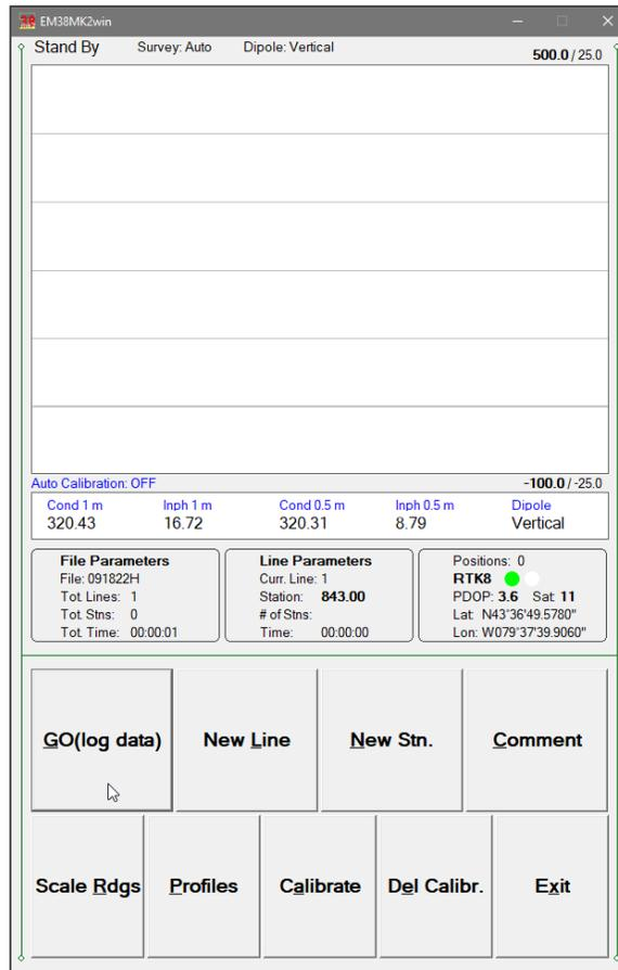
The main portion of the screen is occupied by the plot area which displays profiles (see Figure below which shows Stand By mode after some data were collected). Scale for conductivity and Inphase is
