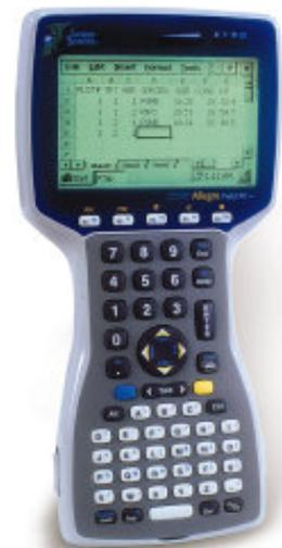
Additionally, and importantly, the Allegro includes two RS-232 serial input connections (and a user-accessible PC card slot) that facilitate the simultaneous collection of both EM and GPS data into a single data file. An optional Trimble Ag114 GPS, providing sub-metre accuracy, is available to support the requirement for position data.
