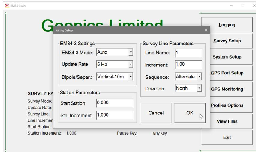
To select any option click on the corresponding drop-down list box or text box, or use TAB key to scroll to the option and then use mouse or the **Down** and **Up** keys in drop-down box (parameters that have only a few possible options), or keyboard for text box entry.
