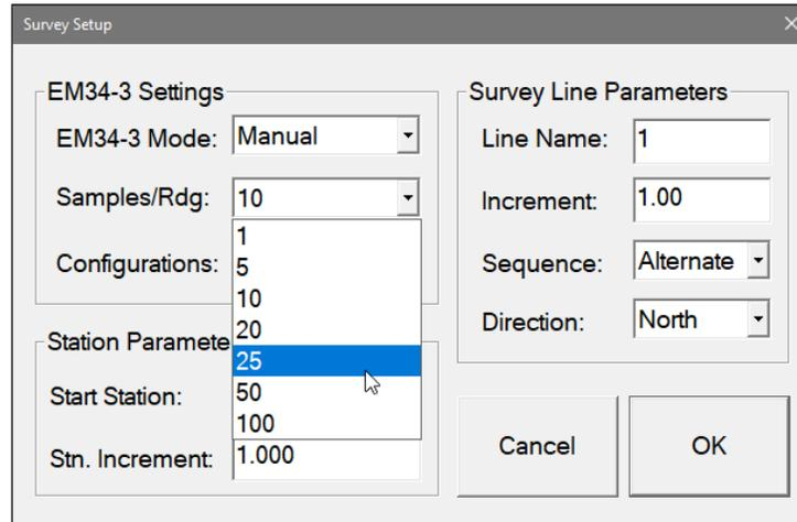
This parameter describes number of readings that will be taken after the trigger switch is pressed. At the end of sampling time the logger will beep and an average value will be written in to the file and plotted on the screen. During the sampling period interval data are measured at approximately 10 readings per second. For example by specifying 10 samples, 1 second will be used at each station. The maximal sampling is 100 readings which corresponds to approximately 10 seconds at each station.
