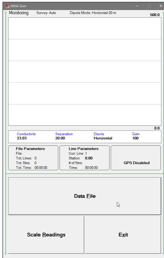
One line of text in the top section provides survey parameters (used in Stand By and Logging modes) and instrument information. In Monitor mode this section displays: current logging session mode (Monitor, Stand By or Logging), survey mode (Auto or Manual), and user specified instrument dipole mode and coil separation. When fiducial marker is pressed then label **Marker** is displayed.
