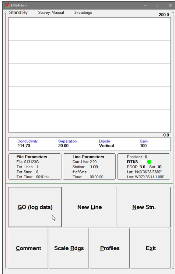
After the screen changes to Logging mode a small label at the top right corner shows how many readings are collected at the station (**Rdg: 0 of 2** and then **Rdg: 1 of 2**) as shown below. Data is recorded in the program memory after the console Record button is pressed. The left Figure below shows action when the first reading is taken (average of total 50 samples) and the Figure on the
