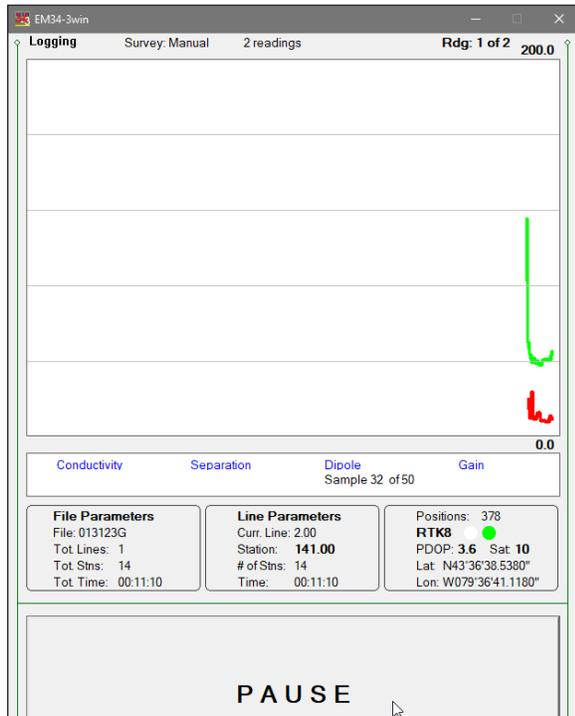
right show the second reading taken. The program keeps track of number of readings (number of Configurations) at each station. It is up to operator to set instrument to desired Dipole Mode and Coil Separation for each reading.
