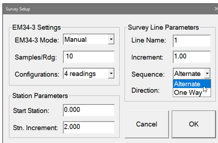
Alternate is used when neighboring lines are surveyed in the opposite direction, which is the most common procedure during field surveys.
