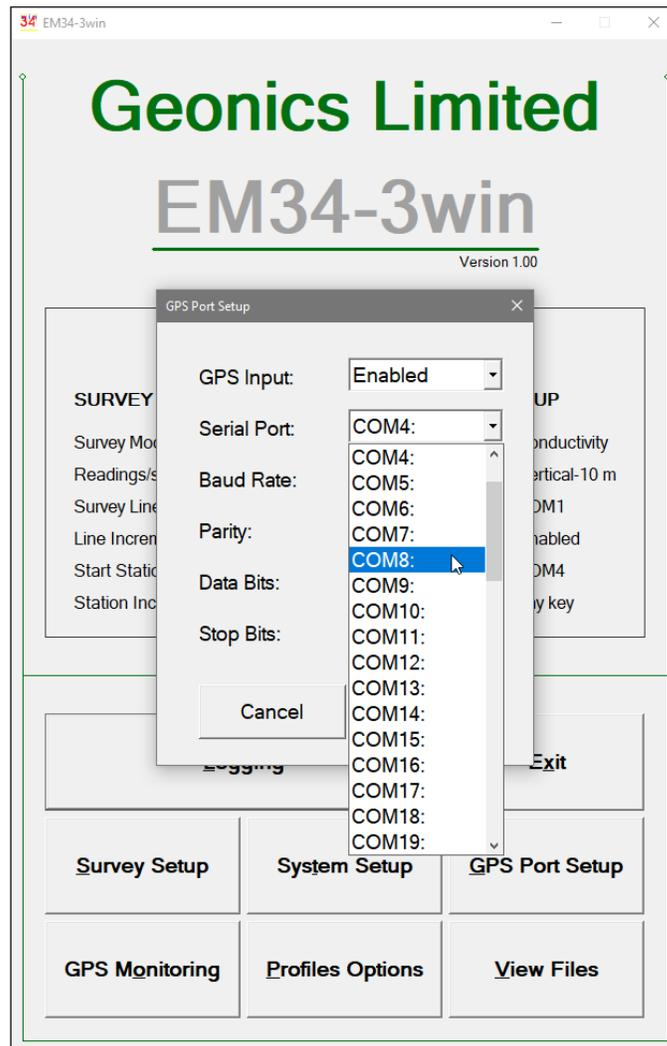
This port must be different than the port specified in the System Setup menu (for EM34-3), otherwise a message will be displayed and ports will have to be reassigned.
