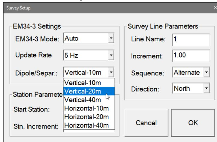
However in Manual mode was selected then any number (up to six) of configurations is available: **1 reading, 2, 3, 4, 5, or 6 readings**. In this case the selected number describes number of different instrument configurations to be taken at each station. Readings at each station can be taken in any order, however care should be taken to collect desired type and number of configurations at each station (Figure below).
