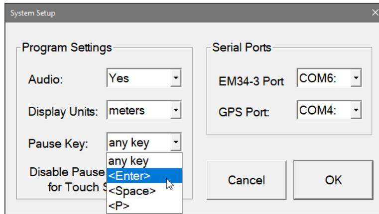
one of the three specific keys for field conditions where a logger key can be accidentally pushed causing unwanted stop of data logging. When Windows based tablet computer Mesa2 is used the best setting is <ENTER> key, since user specified keys P1, P2, and P3 may have various assignment, and when <any key> is selected then only four arrow keys and Enter key are reliable.
