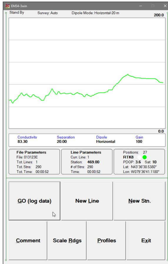
label. Readings are followed by current coil separation (10, 20, or 40 m), dipole mode (Vertical or Horizontal) and EM34-3 currently set range (labeled **Gain**). EM34-3 readings (in numeric form) are updated in Stand By mode approximately 10 times per second. Profiles in the plot area are updated only during Logging mode when data are actually saved in the data file.
