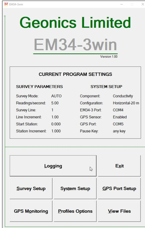
levels, and GPS parameters can be quickly examined and some functions (creating data file, setting scale for profiles) can be performed. After a data file is created in Monitoring mode, the program switches to Stand By mode and allows access to Logging mode. In Stand By mode instrument output can be monitored and some survey and logging parameters can be changed. The Logging mode is used only to record data. Two modes Stand By and Logging are toggled by **GO** and **Pause** buttons.
