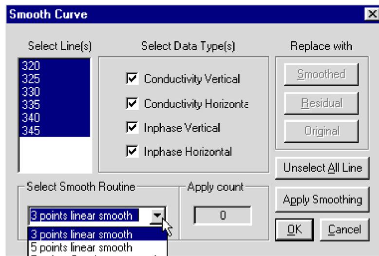
Figure 5.13: The Smooth Data window with list of available smooth functions.
