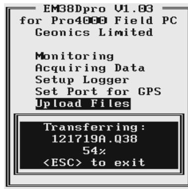
**Figure 3.20:** Pro4000 screen during data transfer
