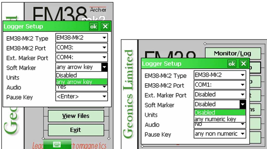
There are two available selections for the Soft Marker: **Disabled** and **any numeric key**. When the latter option is selected pressing any numeric key (from 0 to 9) on the Allegro CX keypad during logging session will tag current station as a station with fiducial marker. It acts exactly the same way as a standard marker located on the instrument panel.
