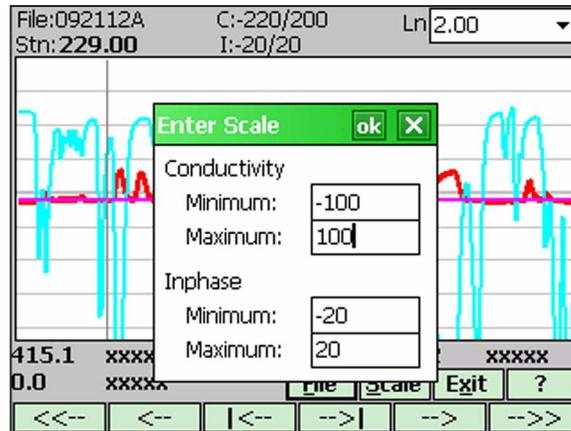
After minimum and maximum values are specified tap the button **OK** or press **ENTER** key to accept new values and the profile plot area will be redrawn (see Figure below).
