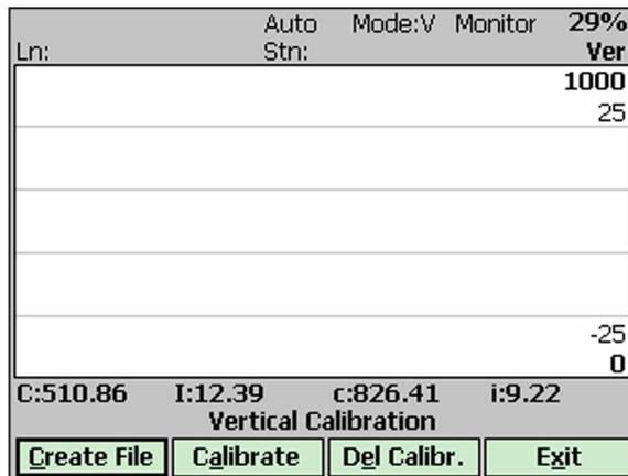
After Vertical calibration is completed (usually few seconds) the program will beep and a message **Rotate to Horizontal mode within 60 seconds** will appear.
