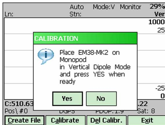
After the instrument is placed on the monopod in Vertical dipole mode tap button **Yes** or press key **Y** (or **Enter** if button is highlighted). After button **Yes** was tapped a messages box disappears and a prompt **Vertical Calibration** is displayed. From now on all messages and prompts will be written under plot section of the screen, in a line that is normally used to display GPS parameters.
