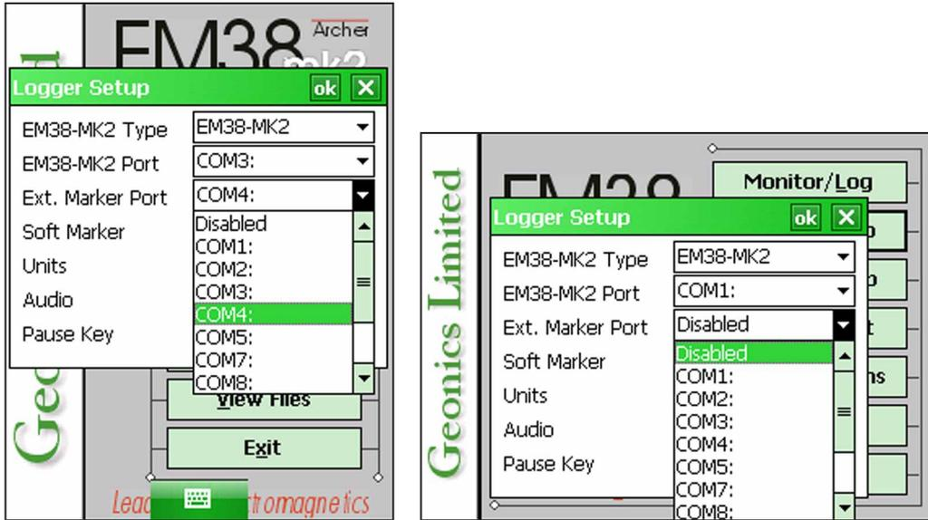
This port must be different than the port specified in the Set Port for GPS option (see next chapter), otherwise a message will be displayed and the ports will have to be reassigned. If External Marker is located on the Extender Arm then The EM38-MK2 and Ext. Marker Port must be the same (usually COM1 or COM2).
