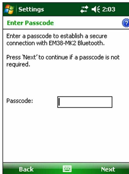
Unless passcode is required (it is not necessary for normal operation) press the Next again and after few seconds a dialog confirming addition of the EM38-MK2 Bluetooth will be displayed (see the top Figure on the next page).
