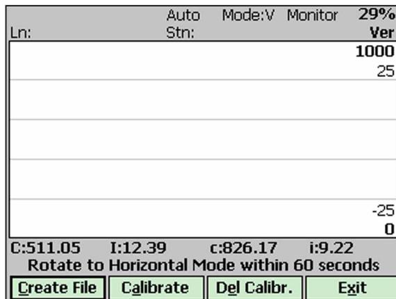
In cases where rotating the instrument takes longer than 1 minute the program will display the message "Horizontal Mode Failed - Wait for Beep", and after a short delay (about 2 seconds) the program will return to normal operation.
