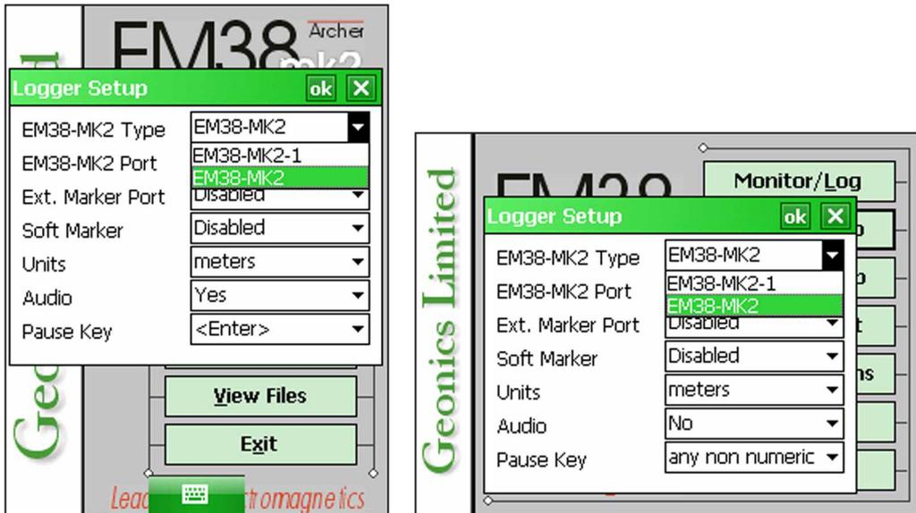
between the models is the number of included receiver coils: the EM38-MK2-1 includes one receiver coil with a 1 meter transmitter / receiver intercoil spacing; the EM38-MK2 includes two receiver coils with 0.5 and 1 meter intercoil spacings. The program default is the **EM38-MK2**.
