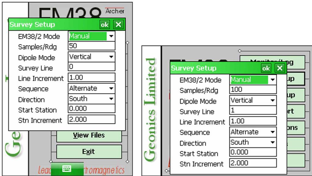
base frequency of the instrument, i.e. user specified frequency of 20 readings/s will result in the effective data acquisition rate of 21 readings/s (every reading is logged), 9 readings/s will cause the program to log at a rate of 10.5 readings/s (every second reading from instrument output is logged), etc. At slower rates the difference between specified and effective frequencies is negligible.
