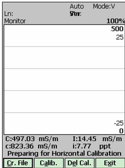
After a small delay required for stabilization the Horizontal Calibration will be performed.
