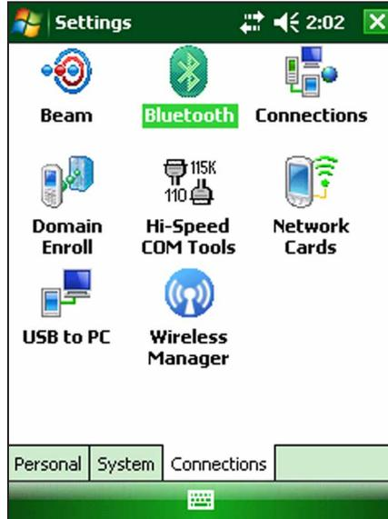
After tapping on the Bluetooth icon the following screen will appear. Tap on the Add new device item. At that time the EM38-MK2 must be ON.
